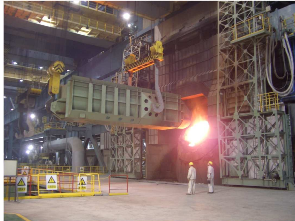
Scrap Chute in Operation
